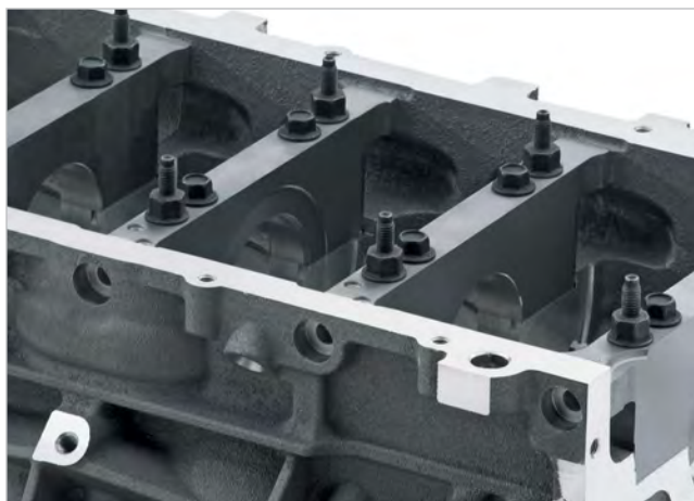
LS1/LS6 5.7L block – aluminum block with 6-bolt main caps A
