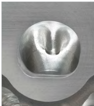
LS3 CNC-Ported Cylinder Head Assembly (combustion chamber) A
