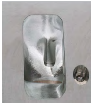
LS3 CNC-Ported Cylinder Head Assembly (combustion chamber) A
