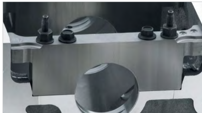
A LS1/LS6 5.7L iron main bearing cap
