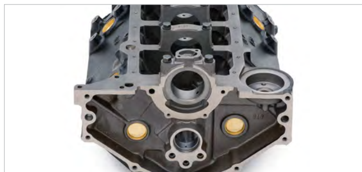
A 305 V-8 Production Block (bottom, rear)
