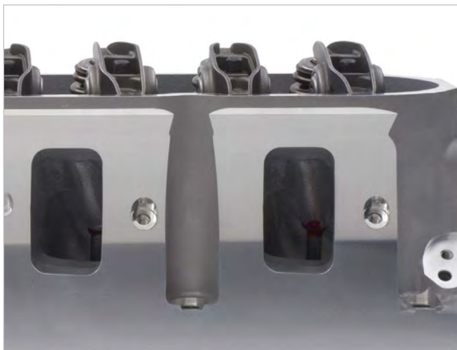
C LS7 Intake Port and Bolt Pattern
