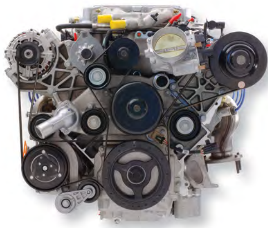
LS9 Accessory Drive System with AC A
