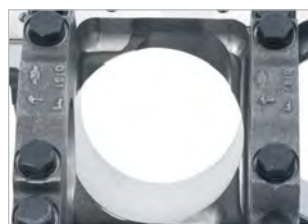
Top: Splayed Main Cap C Bottom: Machined Bottom (close-up)
