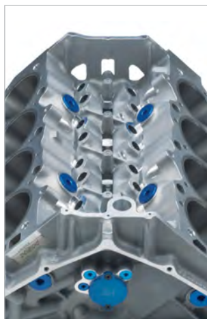
▲ ZL1 Aluminum Big-Block, B Lifter Valley
