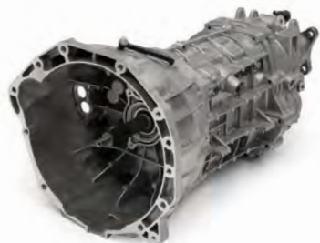
19328976 LTG 4-Cylinder 6-speed Manual Transmission Page 355
