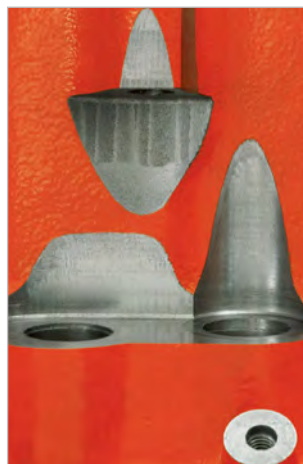
▲ A Machined Lifter Valley Detail
