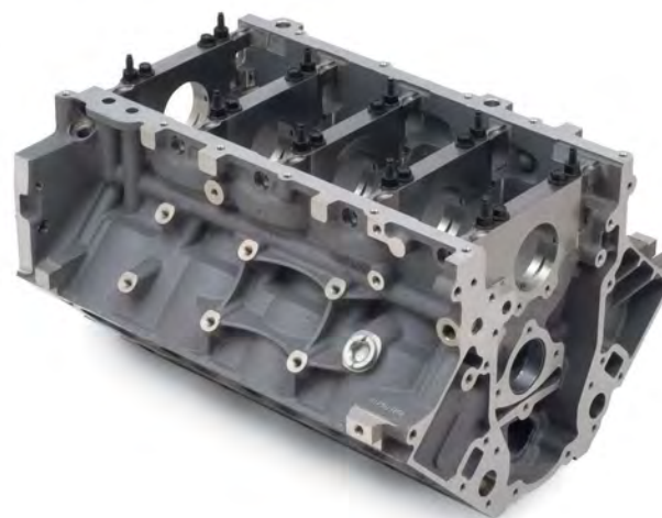
▲ A LS7 7.0L Corvette Bare Block (bottom, front)
