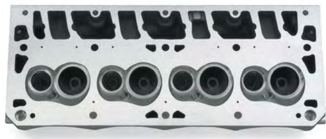
Bare C5R Racing Cylinder Head (combustion chamber) B
