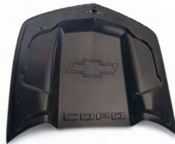
▲ B COPO Camaro Cowl-Induction Hood (Underside)
